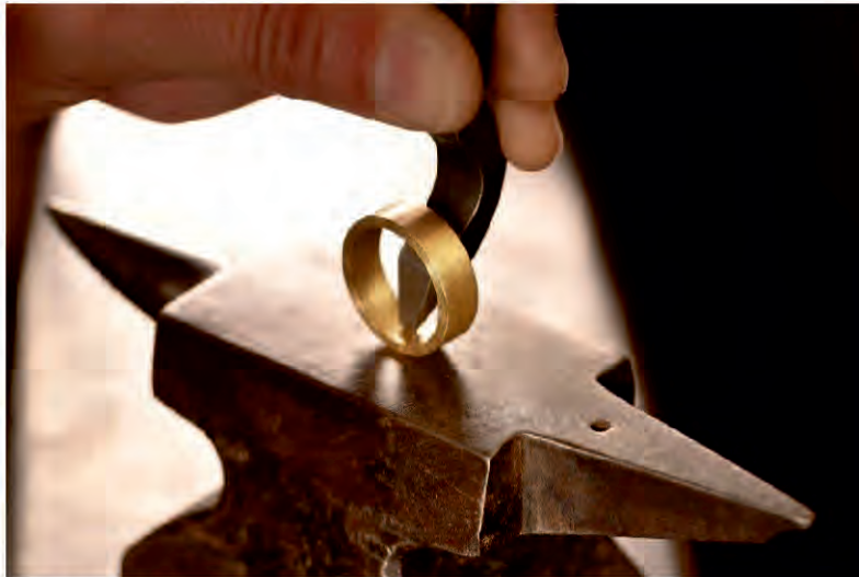
Fig. 1.2.4: A goldsmith punches a hallmark into a golden ring on an anvil
