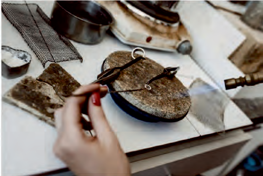
Fig. 1.2.16: Soldering of a silver earring with a flame from a welding torch
